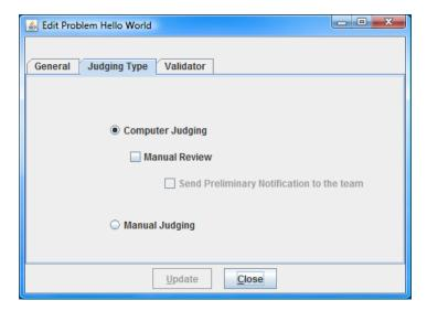
Problems which are configured for computer judging require having a "Validator" associated with them. A Validator is typically a separate user-written program that accepts as input (from  $PC^2$ ) the execution output of a team's run, and returns to  $PC^2$  an indication of what judgment should be applied to the run. [Note that validators have been supported in  $PC^2$  since Version 8.5. However, in
